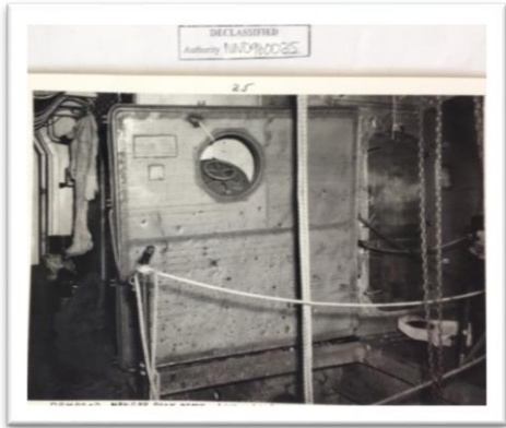
Figure 6-CV5 quick acting scuttle in a watertight hatch (photo from NACP)
