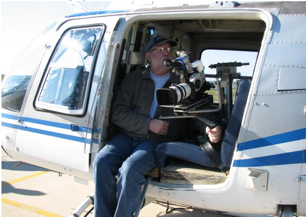
Figure 3. The video camera was attached to a spring-loaded, counter-weighted support on the left side of the helicopter.
