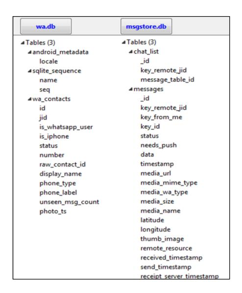
On looking into the files using 'sqlitebrowser' software, we noticed the structure of the database. Please refer to Figure 4. SQLite Browser – msgstore.db -messages table.
