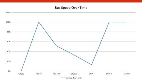
Figure 8.1.2: Transfer Bandwidth Increases Over Prior Generations
