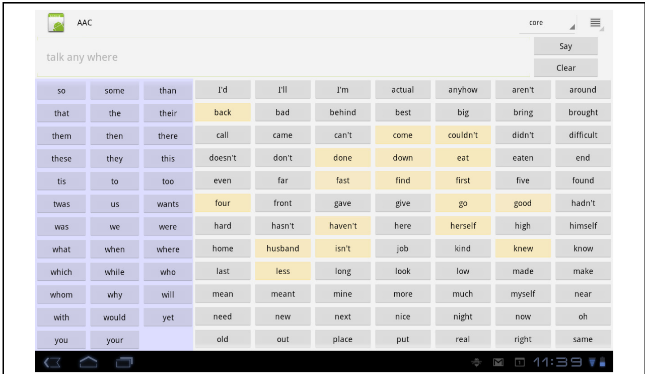
Figure 5. View of the prototype interface after word usage data has been created. The highlighted words have been computed as relevant to the current LexicalContext .
