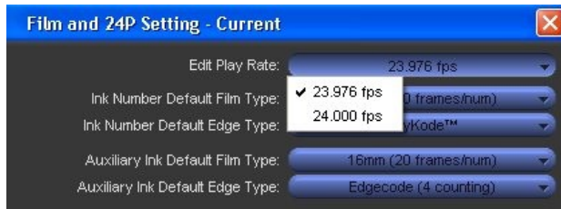
Figure 11. Adjusting the Edit Play Rate for NTSC compatibility.
