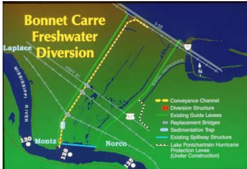
Figure 5. Bonnet Carré Diversion Structure Map (USACE 2003).
