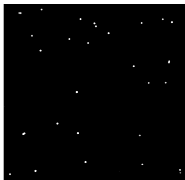
Figure 6.2. Digital fluorescence image of 2.1 \mu\text{m} zinc sensitive lipobeads. Light source: 100W mercury lamp. Excitation filter: D480/30X; Dichroic mirror: 500nm; Emission filter: BA 515nm. Objective: 20X with N.A= 0.5. Neutral density: 1.0. Exposure time: 0.5sec. The imaging conditions remain the same through the experiments unless otherwise stated.
