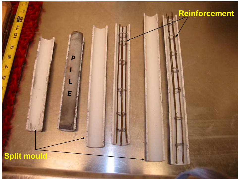
Figure 20. Split moulds used to cast the circular piles. [After Nataraj et al., 2004]
