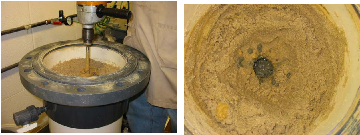
Boring using a drill to cast the cast in situ pile (left); pile after it was cast (right).
