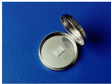
Figure 3.4: Self-powered computer chip in an iButton
