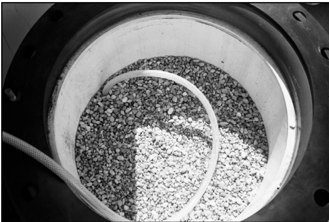
Picture 14 – Lysimeter Prepared to Receive Concrete Weight (after final pea-gravel layer was placed in)
