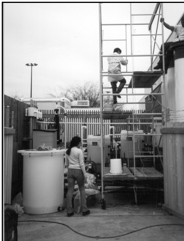
Picture 8 – Arrangement for Filling Lysimeters
