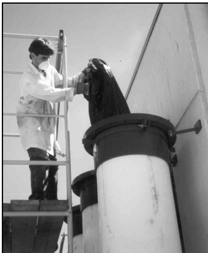
Picture 10 – Filling Lysimeter with Synthetic MSW
