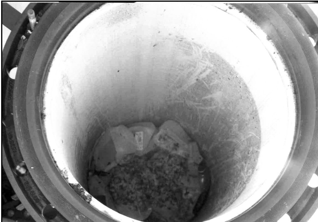
Picture 11 – Synthetic MSW Inside Lysimeter after Manual Compaction
