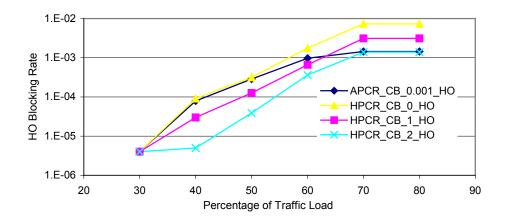
Figure 11. HO Blocking Rate of adaptive PCR\_CB (APCR\_CB) Scheme and HPCR\_CB scheme vs Traffic Load
