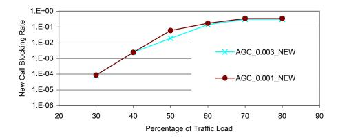
Figure 18. New Call Blocking Rate of AGC Scheme with Different Threshold vs Traffic Load
