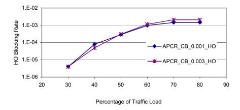
Figure 19. HO Blocking Rate of APCR\_CB Scheme with Different Threshold vs Traffic Load
