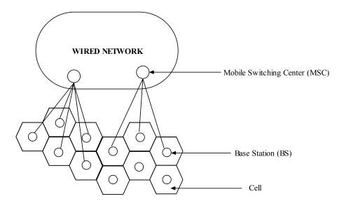
Figure 1. Architecture of cellular networks [12]
