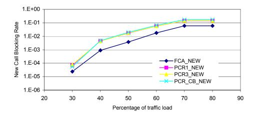
Figure 6. New Call Blocking Rate of Various PCR Schemes and FCA Scheme vs Traffic Load
