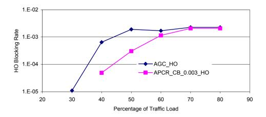
Figure 15. HO Blocking Rate of AGC Scheme and APCR\_CB Scheme vs Traffic Load (handoff blocking threshold is between 0.0005 and 0.003)
