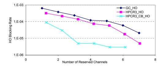
Figure 7. HO Blocking Rate of Various HPCR Schemes and GC Scheme vs Traffic Load
