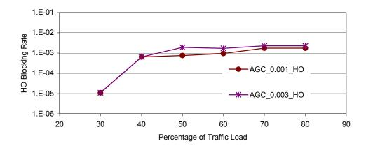
Figure 17. HO Call Blocking Rate of AGC Scheme with Different Thresholds vs Traffic Load
