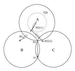
Figure 2. The process of handoff [12]
