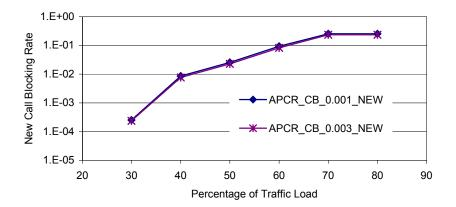
Figure 20. New Call Blocking Rate of APCR\_CB Scheme with Different Threshold vs Traffic Load
