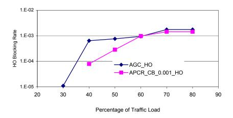
Figure 13. HO Blocking Rate of AGC Scheme and APCR\_CB scheme vs Traffic Load (handoff blocking threshold is between 0.0005 and 0.001)
