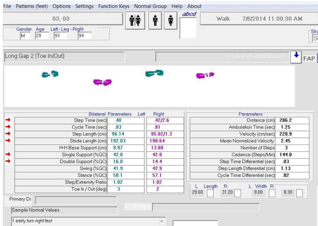
Figure 28. Decrease in left H-H BOS observed on the Gaitrite display when approaching a right step-turn in a young adult male after being cued-early at fast-speed. The gait progression is from left-to-right with the penultimate footfall being the final recorded footfall. The narrowing in left BOS likely contributes to regulation of ML COM acceleration, and the left-ward diagonal body displacement prior to turning right-ward may aid to systematically preserve a ML safety envelope between the turn-execution swing footfall and the right corner hazard cone at the entrance to the turn-zone. The left BOS narrowing may initiate disequilibrium into the right-turn direction, and potentially pose a risk for tripping over one's own feet prior to turning.
