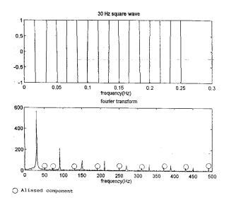
Figure 1. A 30Hz synthesized square wave and its frequency spectrum.
