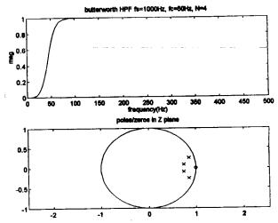
Figure 3. The frequency response and the geometry of the poles and zeros in abutterworth HPF.
