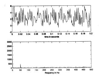
Figure2. A noisy 50Hz synthesized sine wave and its frequency spectrum.
