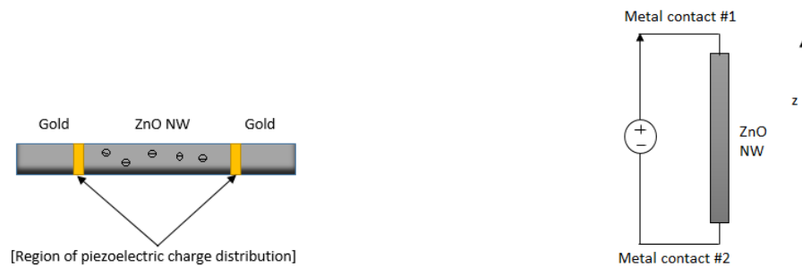
FIGURE 2.1: Schematic of n -doped ZnO NW transistor
