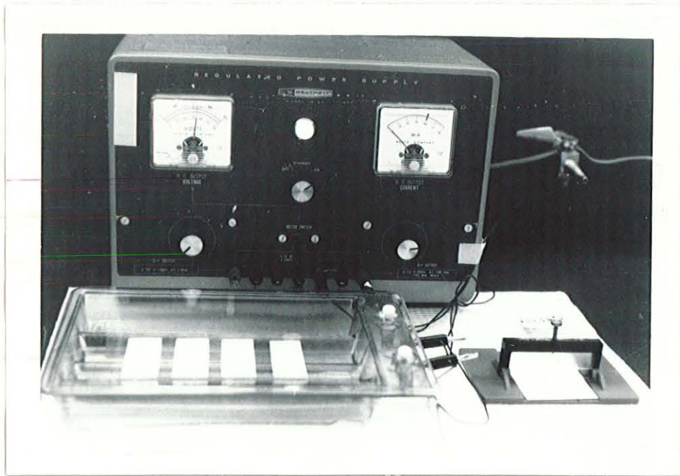
Figure 10.-- Electrophoresis power supply, cell and applicator set up.
