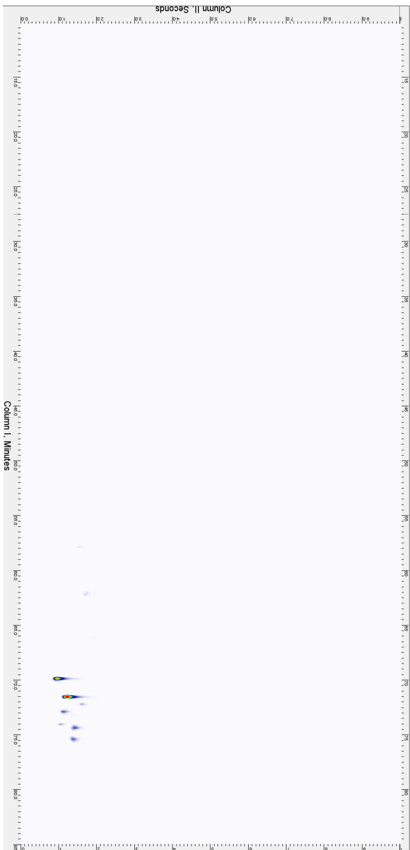
Supplemental Figure 6.4 GCxGC/MS Electron ionization EIC for C_nH_{2n-1}S_N (consistent with alkyl carbazoles) for the Toluene Extracted Fraction of Attapuligus Clay Used for Treating Jet Fuel
