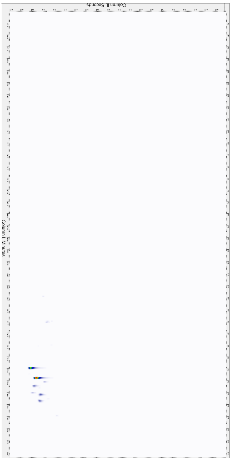
Supplemental Figure 6.8 GCXGC/MS Electron ionization EIC for C_nH_{2n-1}S_N (consistent with alkyl carbazoles) for the DCM Extracted Fraction of Attapulugus Clay Used for Treating Jet Fuel
