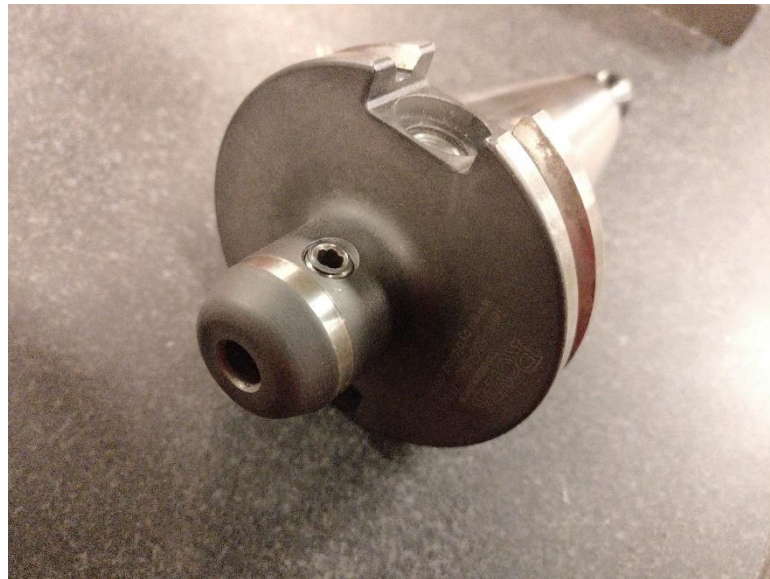
Figure 35. Cat 40 Taper Tool Holder with 6.35 mm diameter hole.
