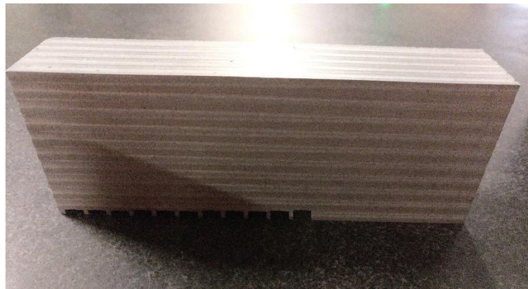
Figure 39. 136.7 mm x 50.3 mm x 26.7 mm AlSiC sample for endurance cutting tests.
