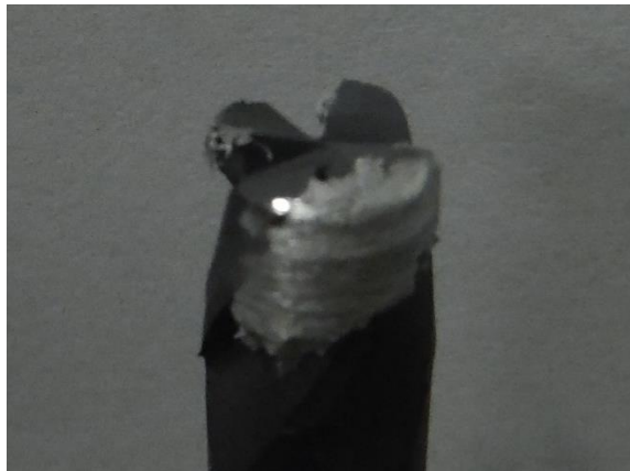
Figure 31. Severe BUE on CVD diamond end mills [17].
