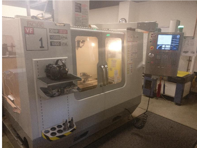
Figure 34. Haas VF-1 CNC vertical milling machine used for all cutting experiments.
