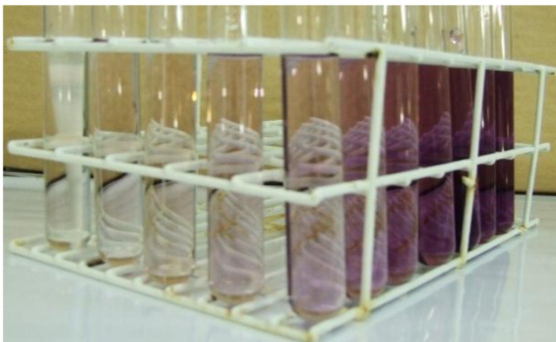
**Figura 11.** Soluções utilizadas para a construção da curva analítica para o AS com solução de Fe (III)  $8,0 \times 10^{-4} \text{ mol L}^{-1}$  e soluções de AS de  $2,0 \times 10^{-5}$ ,  $4,0 \times 10^{-5}$ ,  $6,0 \times 10^{-5}$ ,  $8,0 \times 10^{-5}$ ,  $1,0 \times 10^{-4}$ ,  $2,0 \times 10^{-4}$ ,  $3,0 \times 10^{-4}$ ,  $4,0 \times 10^{-4}$ ,  $5,0 \times 10^{-4}$ ,  $6,0 \times 10^{-4}$  e  $7,0 \times 10^{-4} \text{ mol L}^{-1}$ .
