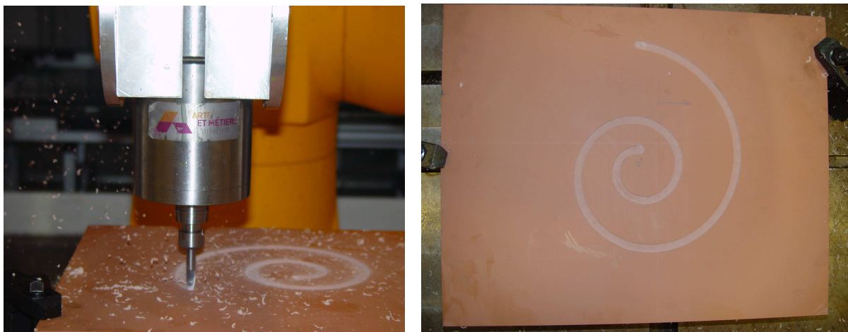
Fig. 14. Machining operations with the robot (cutting depth of 3 mm in resin material).
