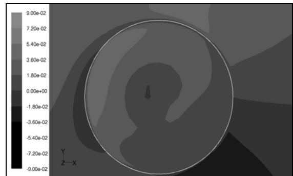
Figure 30. Tangential Velocity- z=0.125D -case III
