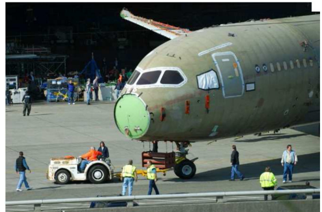
Fig. 8. Forward pressure bulkhead on a civil aircraft being assembled.
