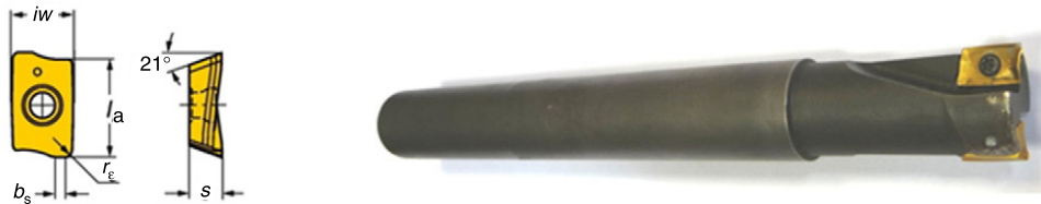
Fig. 2. Sandvik Coromant inserts (left) and tool body (right) used for the tests.
