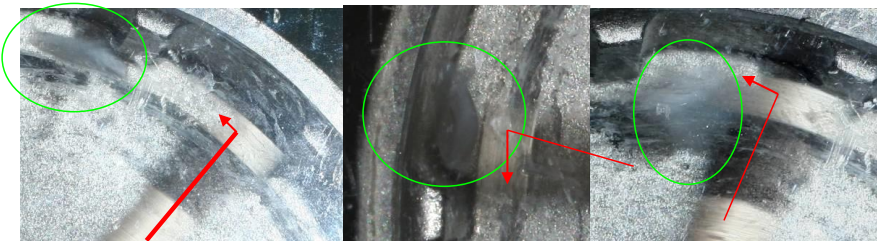
Figure 10: Impact point of (a) particle not fragmented after the first hit, (b) percussion followed by partial fragmentation, (c) grinding followed by total fragmentation of the particle.
