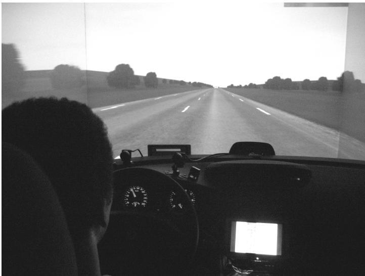
Figure 1. Illustration of simulator setup, showing the FCW system displaying an alarm (red bar) and the secondary task interface (on the bottom right)
