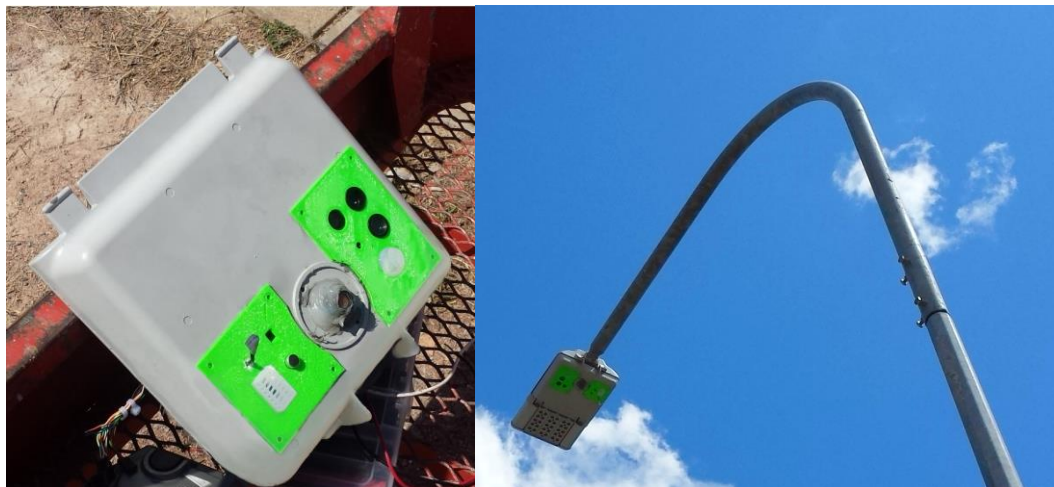
Figure 5.6 - Mounting configuration of testbed sensors. (Left) Traffic sensors are located on the rightmost plate and environmental sensors are located on the leftmost plate. (Right) The mounting plates aimed the sensors at the roadway below.
