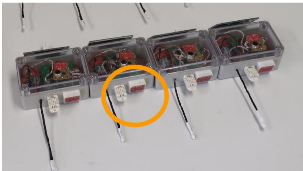
Figure 4.7 - Underside of the deployed sensor nodes, showing the mounting configuration of the humidity and non-contact temperature sensors
