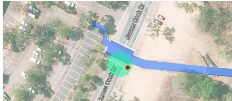
Figure 5.5 - Location of streetlight-mounted test bed showing detection area, pedestrian walkways, and raised crossing
