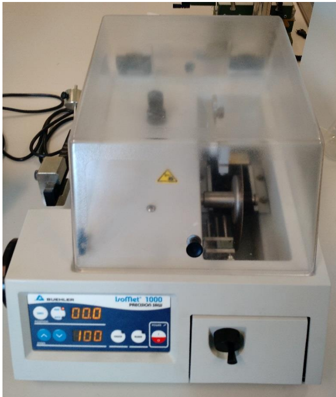
Figure 2-1 Precision saw used for sectioning teeth and preparing dentine blocks.
