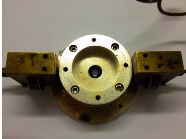
Fig. 5.2 Inner structure of a 25GHz Hakki-Coleman resonator used in this thesis, with one of the endplates removed (photo by the author).
