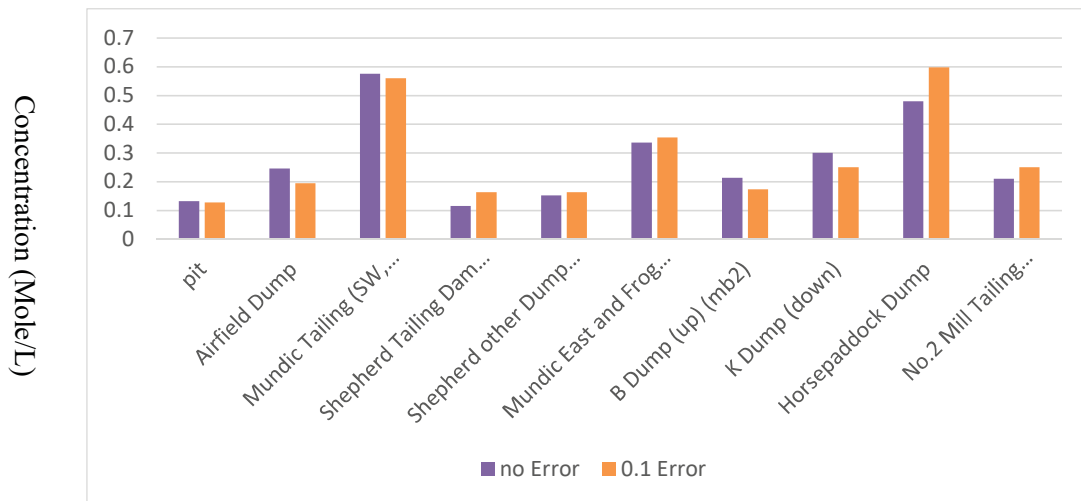
Figure 4.7 Best estimation of concentration (Mole/L) in distributed sources with GP based linked optimization model with actual field data
