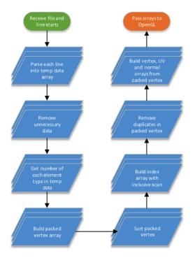
Fig. 3 Reading and parsing stage.
