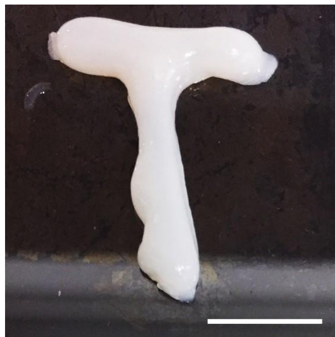
Figure 3.20 - 3D printed structure of CTNW (2.7 % wt.):alginate bioink (top view) Scale bar: 1 cm.
