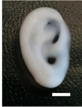
Figure 1.3 - 3D printed ear using a bioink composed by alginate sulfate and nanocellulose. Scale bar: 5 mm. Image adapted from [11].
