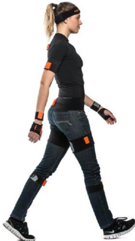
Figure 3.1 | Example of an individual outfitted with Xsens wearable inertial sensor technology: (1 ×) on head, (1 ×) on chest, (2 ×) on arms, (2 ×) on forearms, (2 ×) on hands, (1 ×) on pelvis, (2 ×) on thighs, (2 ×) on legs and (2 ×) on feet [70].
