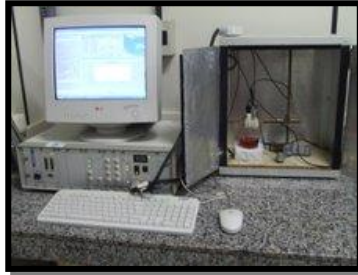
Fig. 1.6 – Potenciostato Autolab GSTAT30
