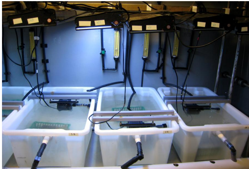
Fig. 4.5 Sediment treatment tanks within the AIMS aquarium facilities. To ensure sediment suspension, pumps were inverted and suspended at the waterline using grey metal bars.
