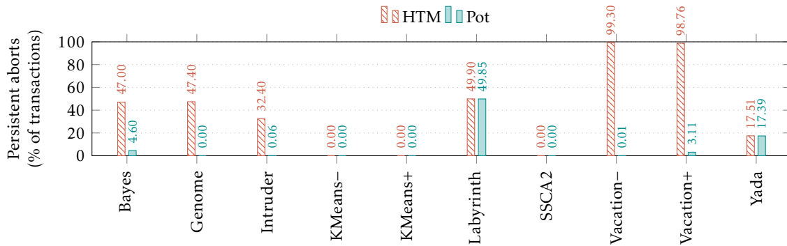
Figure 3.13: Percentage of transactions that experience persistent aborts using baseline HTM transactions and Pot fast HTM transactions on the STAMP benchmarks (lower is better). – and + refer to the relative levels of contention in the configuration.
