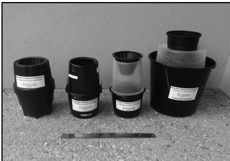
Fig. 1. MosquiTRAP, double sticky ovitrap, small Gravid Aedes Trap (GAT) and standard large GAT used in the field trials. A 33 cm ruler is provided for scale. The large GAT is the standard used in most field trials.
