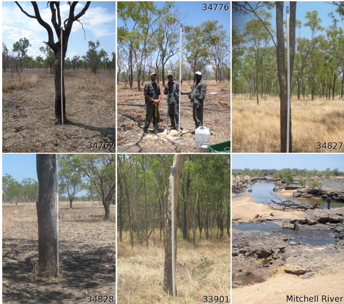
Figure 5.11: Capacitance loggers set up in the Mitchell floodplain (as numbered). The main channel of the Mitchell near Shelfo Station is shown in its dry season state in the lower right-hand image
