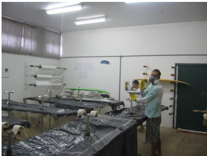
FIGURA 15 – Laminando as pranchas
