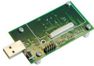
Figure 2.4: MIB520 USB Interface Board [35]
