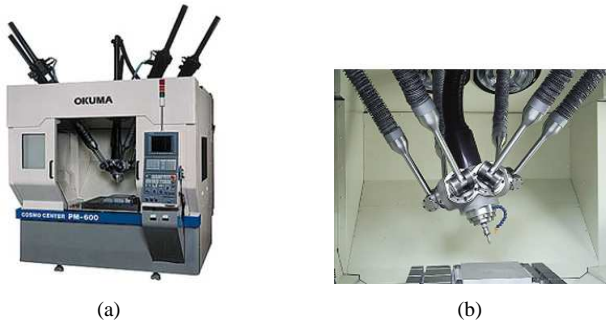
Figure 87 – 5-axis machine: (a) Okuma Cosmo Center PM-600 (GMBH, 2009; BONEV, 2009a). (b) detail of its platform (BONEV, 2009a).
