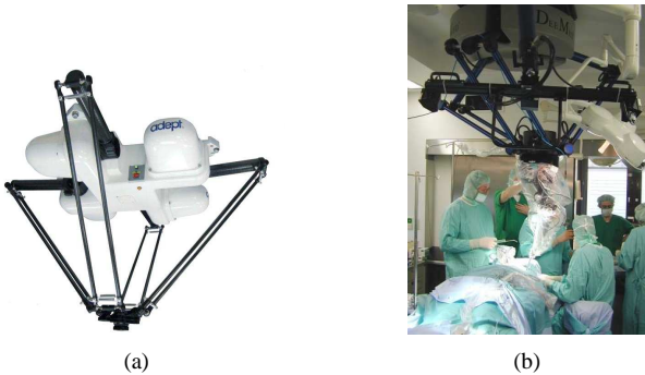
Figure 83 – Delta-type robot: (a) Adept Quattro s650H (ADEPT ROBOTICS, 2009). (b) World's first Craniomaxillofacial surgery using a Delta (LUETH, 2009).
