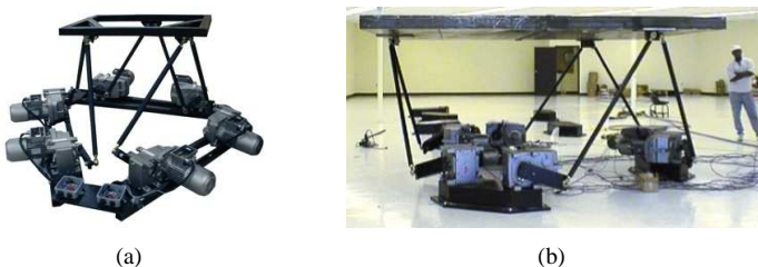
Figure 89 – Hexa 710-6 from Servos & Simulation (SERVOS AND SIMULATIONS, 2009): (a) Detail of actuation. (b) An application of the Hexa as an entertainment simulator motion base.
