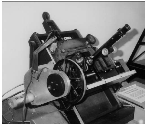
Figure 6: A Gaertner measuring engine, like the one used by Millman (courtesy: McCormick Museum).
