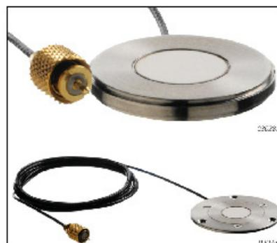
Designed for use on airplane surfaces during in-flight testing, as well as in wind-tunnel testing and other, similar applications, Surface Microphone Type 4948 is a rugged and stable measurement microphone. The microphone housing and the metallic parts of the diaphragm-backplate arrangement are all titanium, ensuring uniquely high resistance to corrosion.
