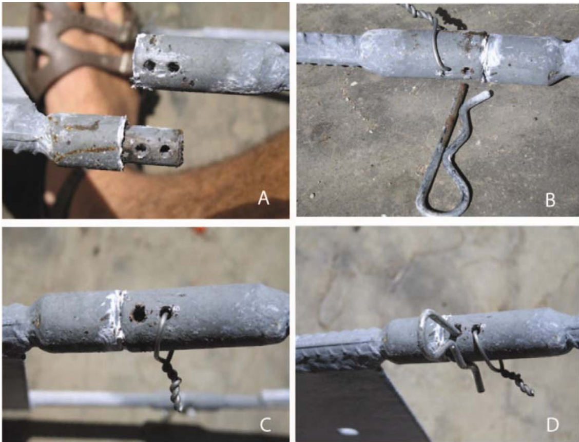
Figure 2.3. The lug and socket in each leg of the frame (A) used #18 gauge (1.25mm) galvanized wire and a B10 'R' Clip to enable (B,C) or bypass the weak-link (D) .
