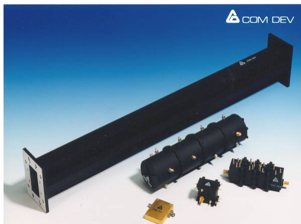
Fig. 1. Filter size comparison: (a) cavity, (b) dielectric, (c) dielectric in superconducting enclosure and (d) microstrip superconducting filters for satellite communication after [2]
