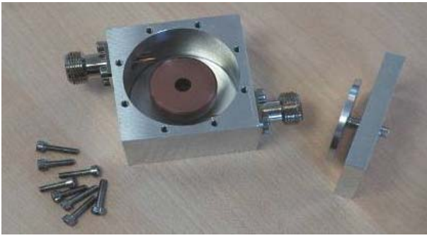
Fig. 2. Dielectric Resonator in a cylindrical cavity
