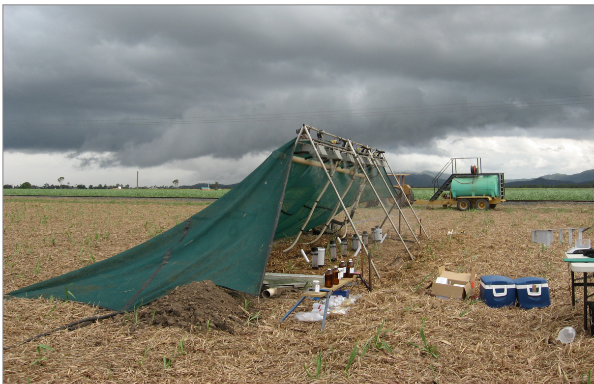
Figure 3: Rainfall simulator set up to investigate proposed sugarcane BMP and resultant water quality outcomes in the Mackay-Whitsunday region (sourced from Masters et al. In prep).
