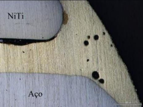
Micrograph showing the interface between NiTi (top) and Aço (bottom) for specimen P.6. The NiTi is a light grey circular area, and the Aço is a darker grey area. There is a distinct gap between them, and several dark, circular spots are visible in the Aço region. |
