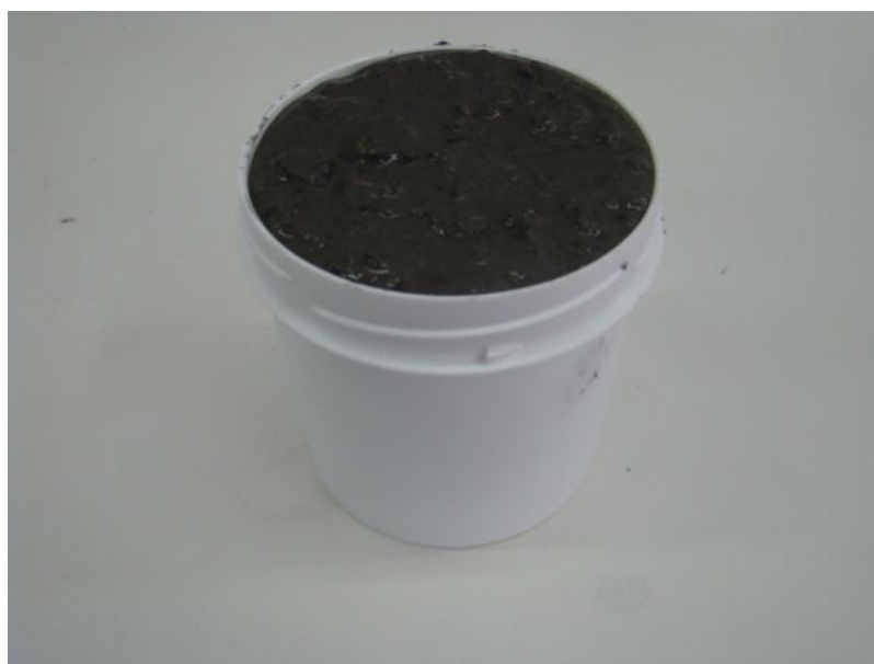
Figura 2.6 – Provette contendo betão fresco ( \varnothing = 7 cm; h = 8 cm)
