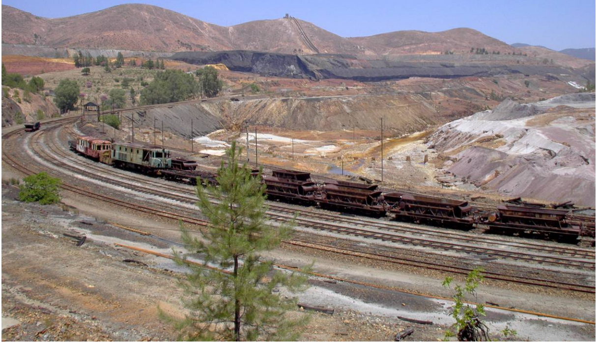
Figure 1: Slag heap, sulfidic waste dumps, and abandoned railway carriages at Rio Tinto, Spain. The mining activities have left uncountable waste rock heaps, ore stockpiles, tailings dumps, slag deposits, and settling ponds, most of which do not support any vegetation. The exploitation of sulfidic ores has created a unique “mining landscape” and caused massive ARD flowing into the Rio Tinto.
