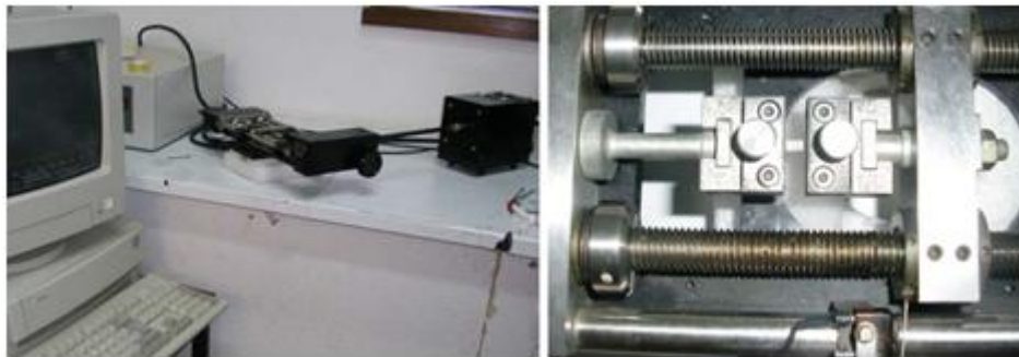
Figure 2.4 – Photograph of the (a) tensile tests equipment and (b) detail of the film sample placed between the clamps.
