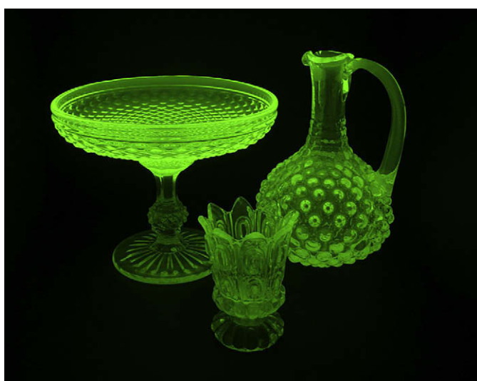
Fig. 2. Uranium glasses from a private collection under UV light (stemmed plate, toothpick holder and oil cruet).
